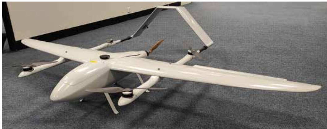
Baby Shark long endurance VTOL drone
